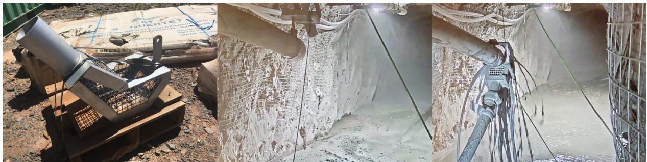
Figure 3 Three photographs showing the catcher on surface, installed but not deployed, and the catcher deployed with CPB flowing through it
